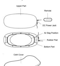
Connect the adapter and DC power Jack of the unit, then connect the power supplier.
