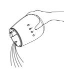
8. Drain and rinse the water tank thoroughly to remove any sediment and dirt.
