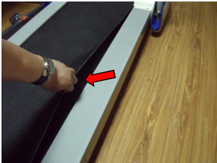
Step 1: To lift up running one edge side then spray in 10ml silicon oil.
