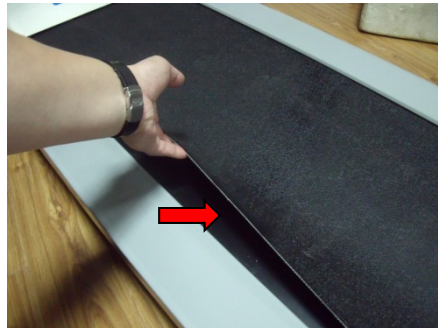
Step 2: To lift up running another edge side then spray in 10ml silicon oil again.
