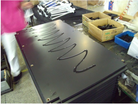
Step 1: pour down 20-25ml silicon oil by "S" track.
